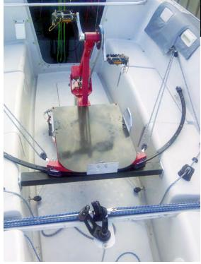
Callahan's special steering system on his Sonar includes a set of bike pedals he uses to steer and a rotating seat.
